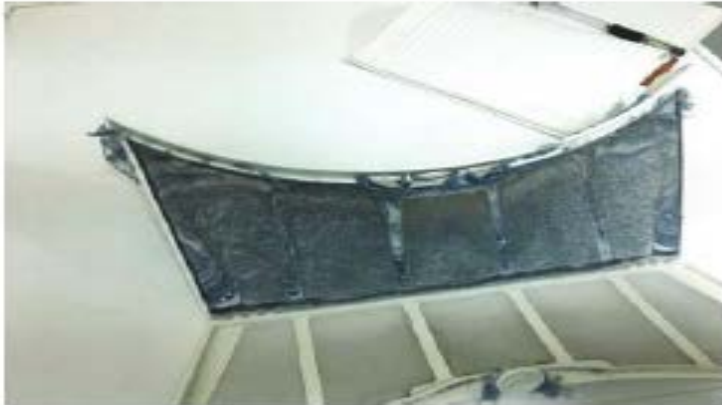
Totally blocked filter of a domestic type tumble dryer
